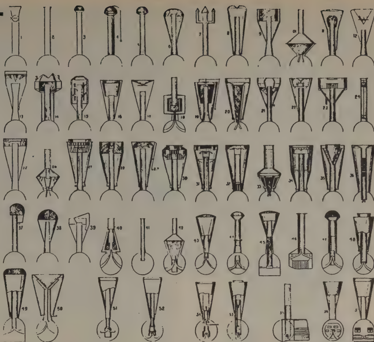
Excess of novelty: American smokestack spark arrestors (1831-57). The smokestack designs depicted here are fifty-seven of the more than one thousand that were patented in the nineteenth century.
